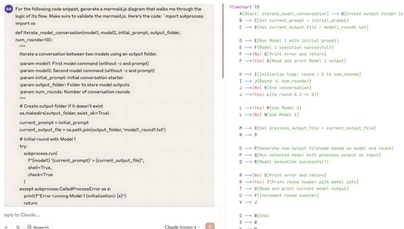
Figure 22. I ask Claude.ai to diagram the flow logic of the code block that puts two models into conversation with one another. It returns the diagram using the conventions of standard Mermaid.js text. A variety of text editors and websites can turn the Mermaid.js text into a chart.
